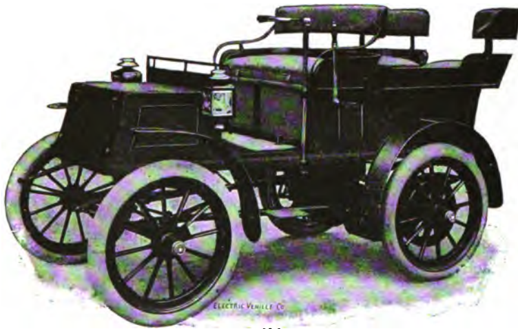
FIG. 446.—"Columbia" Electrical Tonneau Carriage. The weight is about 2,800 pounds; the travel radius, about forty miles per full charge of battery; the maximum speed, thirteen miles per hour.
